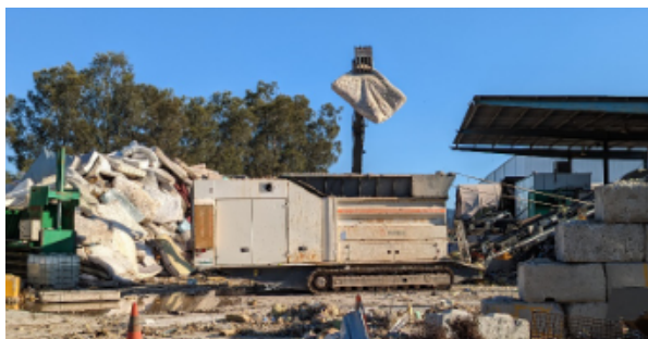
Figure 2. End of life mattresses showing pocket springs and mechanised shredding.
